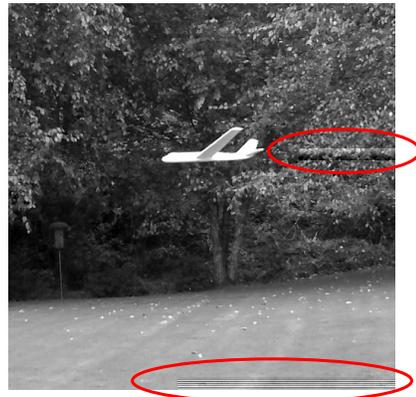
Fig. 8. Intra encoded frame with spatially propagating errors
